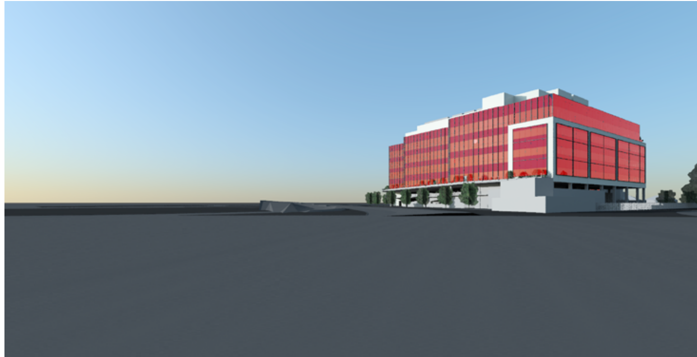
Area of Glazing that will have visible reflections in Red - see annual graph
